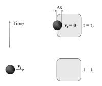
Figure 6.3: A massive plastic block is deformed when hit by a ball moving by inertia. Traditionally, it is stated that the ball's kinetic energy converts into a deformation energy. However, a deep physical explanation reveals that the ball's energy is inertial energy since the deformation is caused by the work done by the real inertial force with which the ball resists its deceleration
