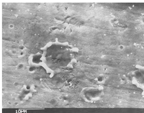
Figure 4 Impact marks of small CPs hitting a titanium target [2]
